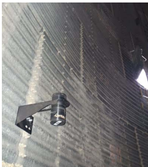
Fig. 11 The three-dimensional model of the cylindrical silo considered in this work Fig. 12 Installation of sensor B inside the silo
